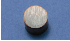
Cu-Bond Round Conductor cross-section
