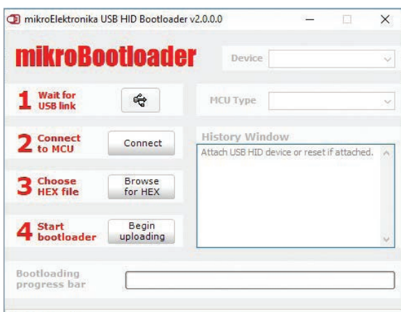
Figure 5: Bootloader PC application software used to upload MGATESTER1 firmware updates.
